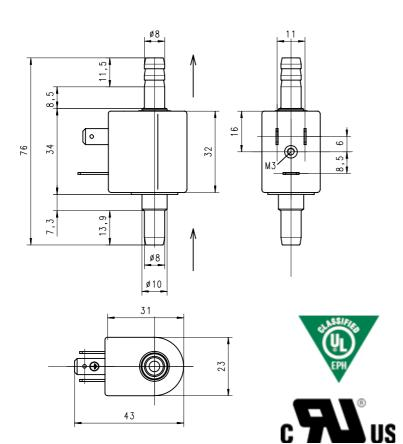
Dimensions in millimeters (mm)
